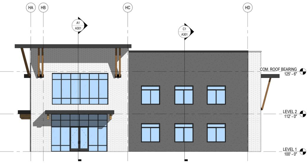
A1 COMMERCIAL BUILDING EAST EXTERIOR ELEVATION
