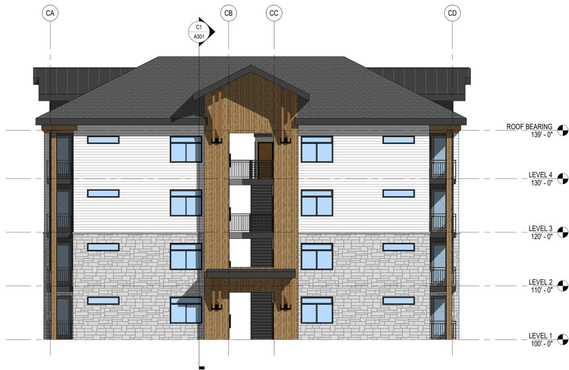
C3 BUILDING C EAST EXTERIOR ELEVATION
