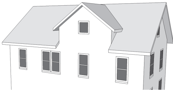
Figure 5.58 - Parallel ridge line with gable example
